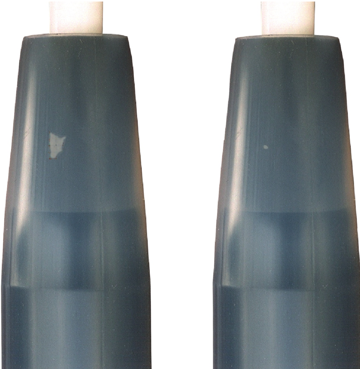
Fig. 3: Disappearance of an air bubble in the gap between the sleeve insulating body and the FSE.
